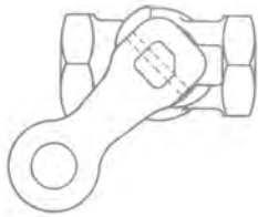
Piece No. 75588 3/8" Cut-out Cock, Complete
