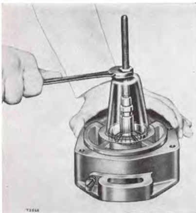
REMOVING MAGNET ROTOR BEARING OUTER RACE
