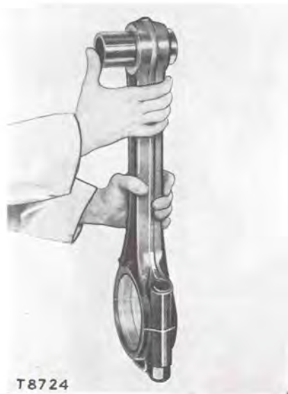
CHECKING PISTON PIN BUSHING
