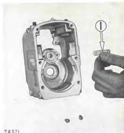
REPLACING BRUSH HOLDING PLATE 1—Brush holding plate.
