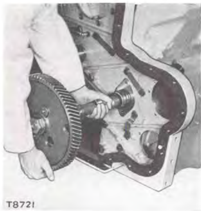
T8721 REMOVING A CAMSHAFT AND CAMSHAFT GEAR
