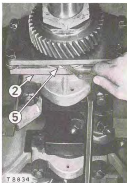
MOVING CRANKSHAFT BACKWARD AND CHECKING END CLEARANCE 2—Thrust plate (rear). 5—Thrust washer.
