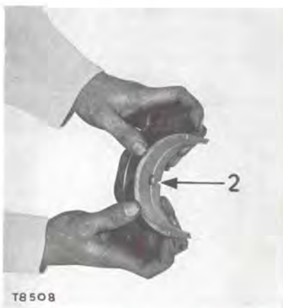
REMOVING BEARING SHELL 2—Bearing shell.
