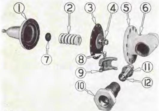
DISASSEMBLY OF PRESSURE REGULATOR
