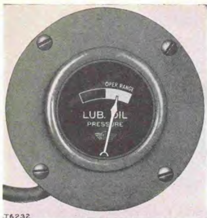
LUBRICATING OIL PRESSURE GAUGE
