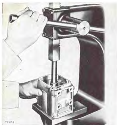
PRESSING IN DISTRIBUTOR ROTOR BEARINGS
