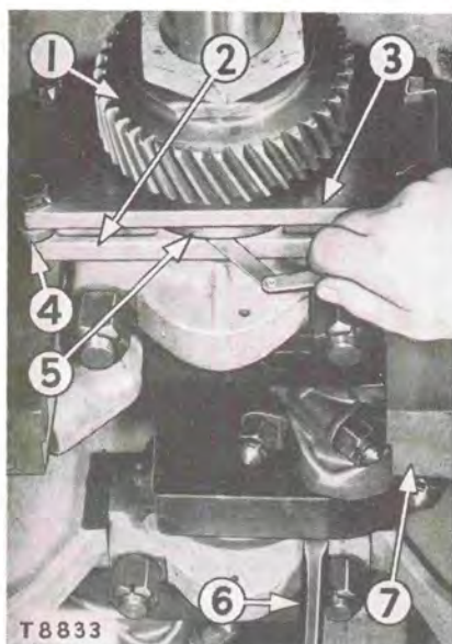
MOVING CRANKSHAFT FORWARD AND CHECKING END CLEARANCE 1—Crankshaft gear. 2—Thrust plate (rear). 3—Thrust plate (front). 4— Spacer. 5—Thrust washer. 6—Pinch bar. 7—Crankcase.
