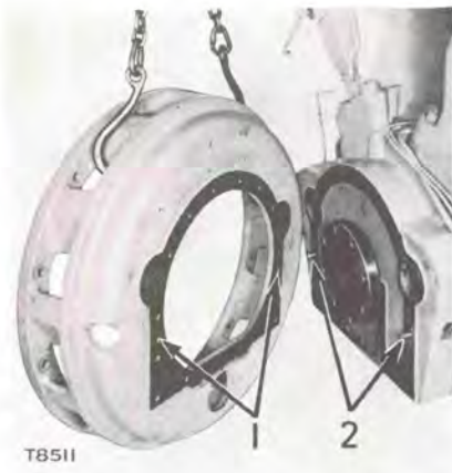
INSTALLING FLYWHEEL HOUSING (D17000L ILLUSTRATED)
