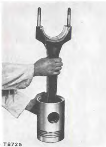
CHECKING PISTON PIN BUSHING
