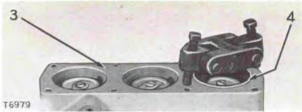
REMOVING RETAINER RING 3—Regulator housing. 4—Retainer ring.
