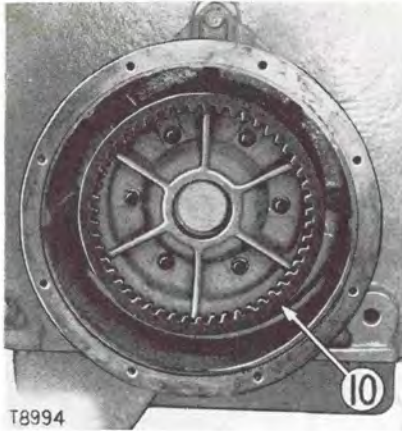
REMOVING COUPLING 10—Coupling.
