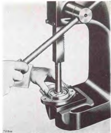
PRESSING OUT MAGNETO ROTOR OIL SEAL
