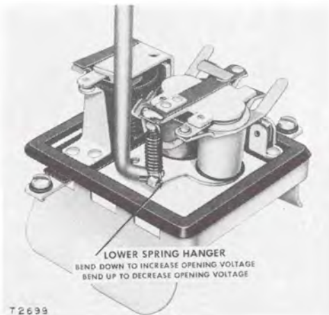
ADJUSTING STEP-VOLTAGE CONTROL OPENING RANGE
