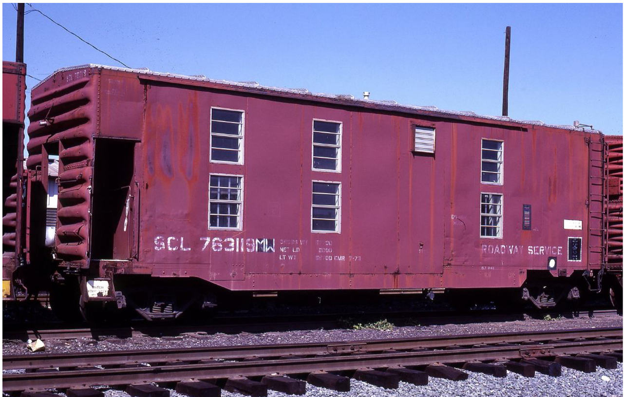
SCL 763119 MW is a former SAL AF-4 which has been converted to a roadway service laborers' car. The 14' door opening has been plated over and jalousie-style windows have been installed to permit some ventilation. The silver roof was applied to aid in heat deflection, and the ends have been cut to permit entry between cars. (Warren Calloway photograph)
