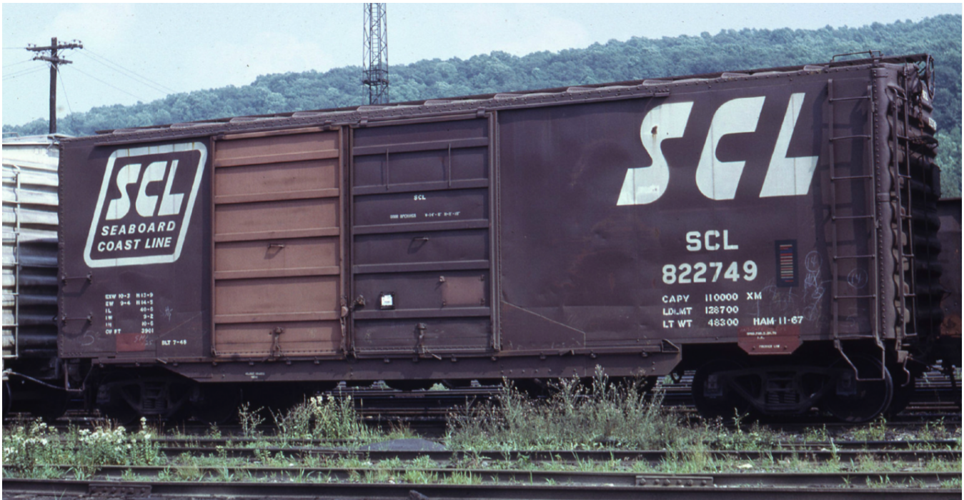
SCL 822749 sits at unknown location, following the SCL merger. This example was repainted in Hamlet, North Carolina in November 1967. The addition of doorway gussets and new 6 panel seven-foot Superior doors marks this car found in general or paper service. The running boards remain intact as well as the as-built ASF A-3 ride control trucks. (Photographer unknown, Justin May collection)
