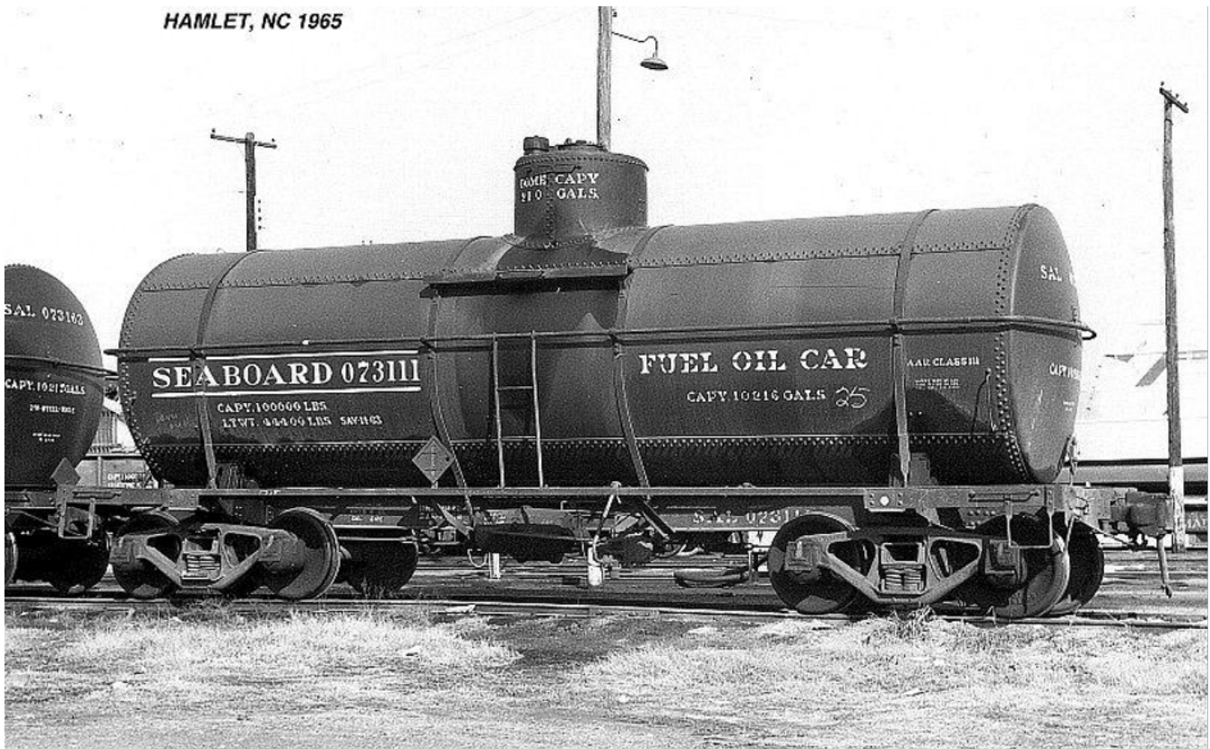
SAL 073111 is another 10,000-gallon example constructed by ACF in 1925-1926. The shell capacity contained 10,216 gallons, while the dome was capable of containing 210 gallons. The car is a former MPLX car which consisted of eight various series, and the original car number is not known. (Warren Calloway photograph taken in Hamlet, NC circa 1965)
