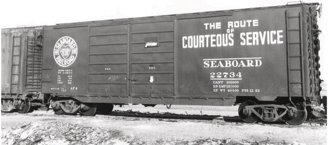
Above: SAL 22734 was photographed in Calexico, California, on January 15, 1955. The variation in car body color and the black ends can be discerned when looking at the B end of the car. The Route of Courteous Service was a standard slogan applied to these cars. SAL 22734 was last reweighed in Portsmouth, Virginia in November 1952. The enlarged door opening best suited these cars to high cubic capacity loads such as automobiles, furniture, and paper. ( Chet McCoid photograph, Bob's Photo ) Below: SAL 22595 was photographed in Acca Yard, Virginia in a much later scheme applied in 1965. The six panel Superior doors are replacement equipment and the car now features a solid boxcar red scheme on the ends and sides. The application of the ACI label and the 50-ton ASF A-3 trucks with exposed roller bearings places this car firmly in the mid-1960s. ( Bob's Photo )
