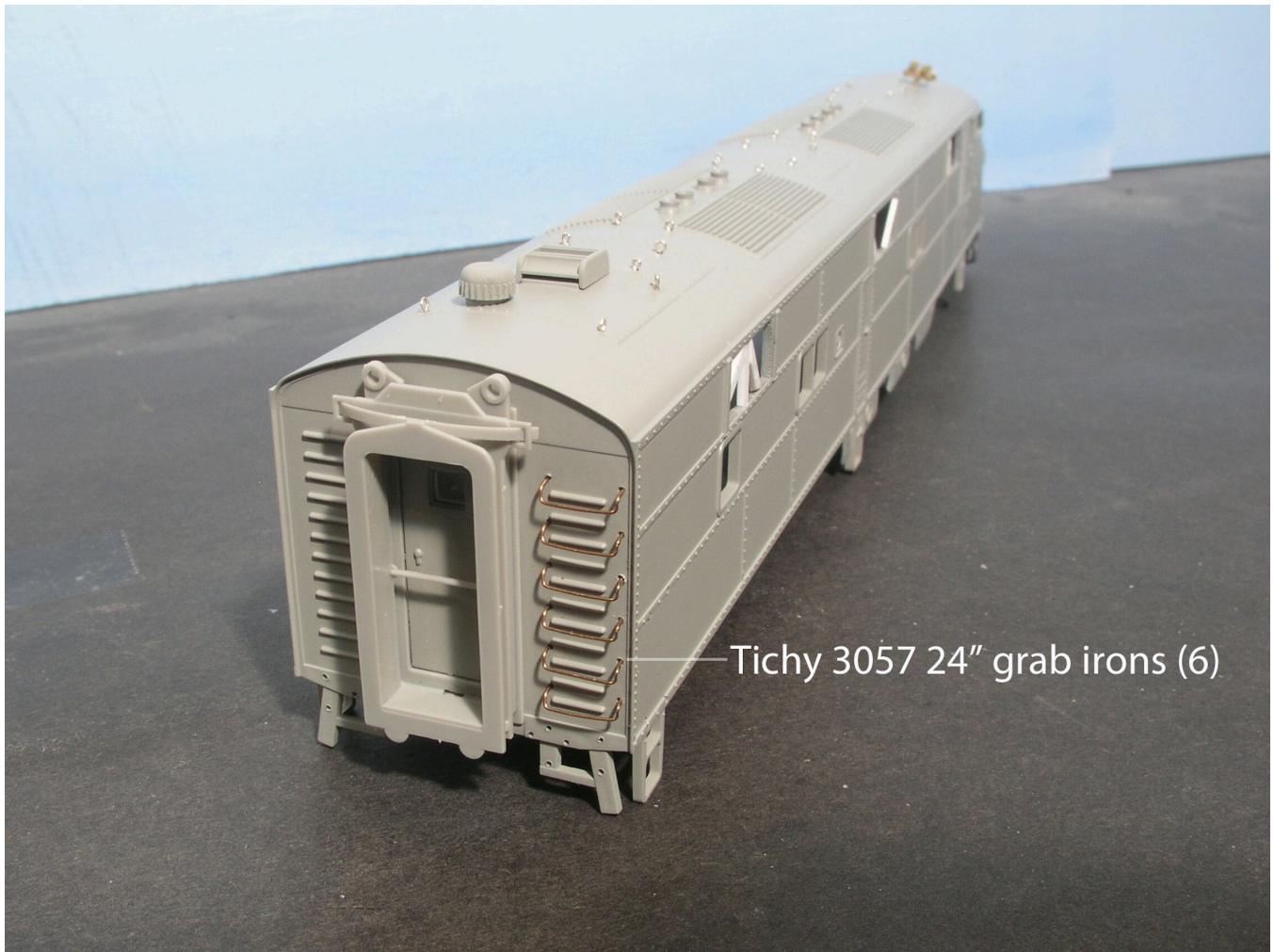
Note the installation of the 24" drop grab irons on the engineer's rear side of the locomotive. The grab irons are installed per the prototype. Additionally, note the location of the "brow" grab irons above the windshields. The dimensions are best located using a digital caliper.
