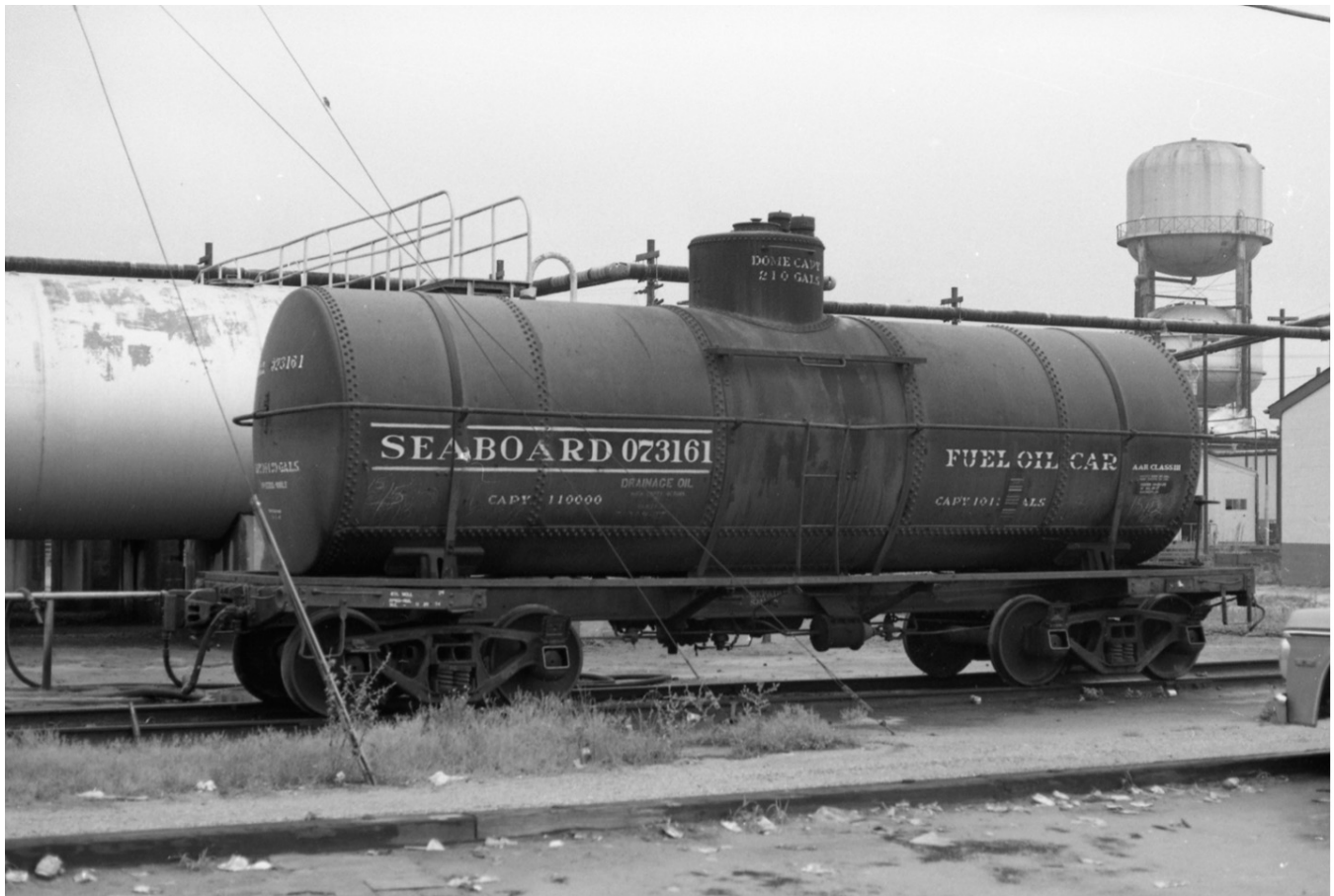
SAL 073161, formerly Mexican Petroleum Corporation (MPLX) 724, is an example of a 10,000-gallon riveted tank car constructed in January 1920 by ACF (Lot Number 8727D). The car uses a gauging table of 4 (0.2242" thickness, 9.146 pounds per square foot). The lack of a pronounced end sill arrangement and inward facing braces denotes this as an ACF product. (Larry Goolsby photograph, Hamlet, NC taken on August 8, 1976)
