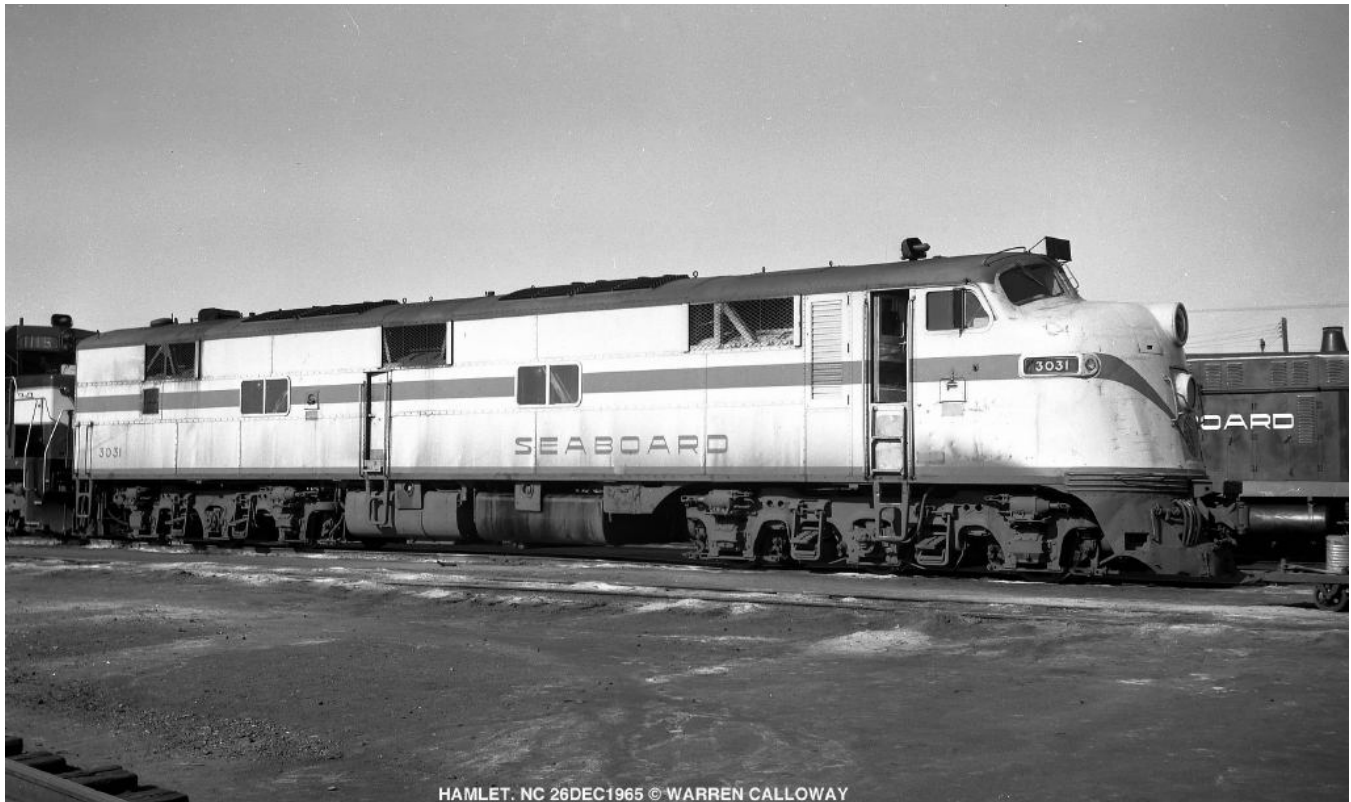
SAL 3031 was built in September 1946 and is seen awaiting assignment in Hamlet, NC nearly twenty years later on December 26, 1965. The weathering and road grime are indicative of the use these E7s saw throughout the 1960s. SAL 3031 is coupled with SAL 1115, a 1964 built SDP35, which were purchased to supplement the aging E unit fleet. (Warren Calloway photograph)
