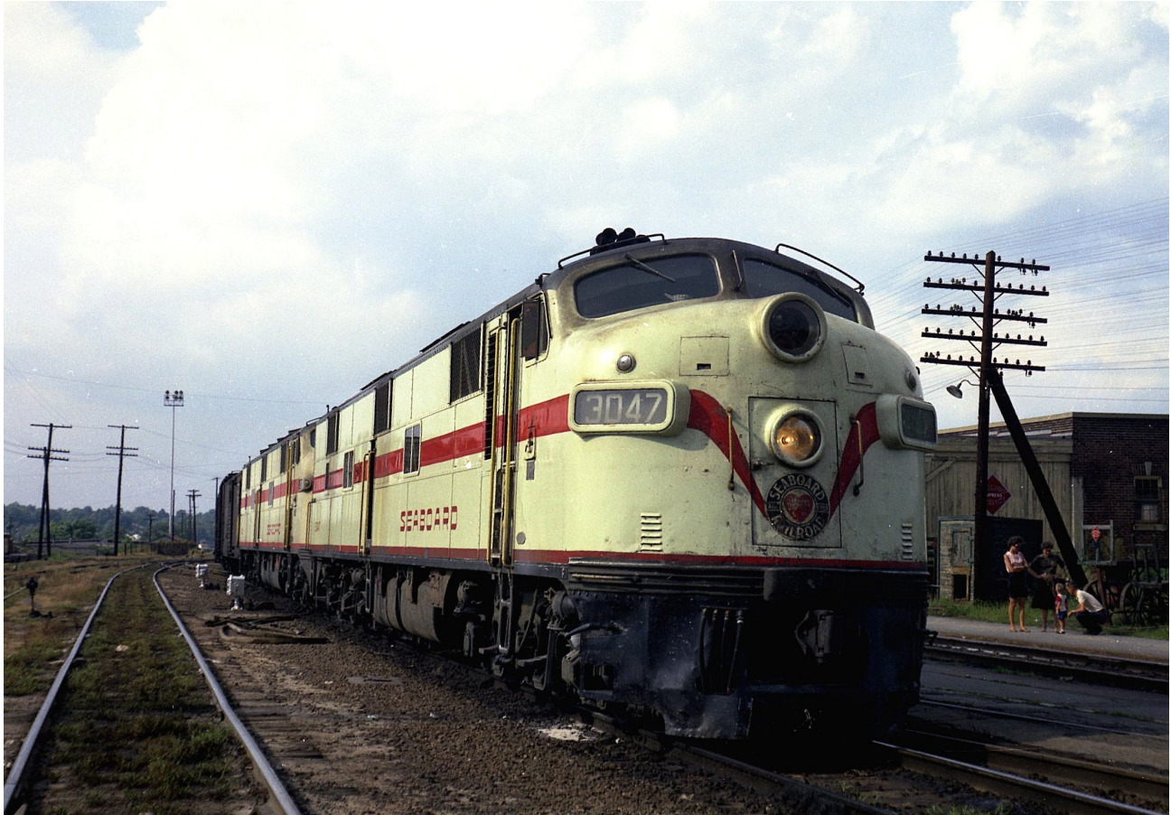
Seaboard 3047 and unidentified E7A are powering Number 3, an express, mail, and passenger train. The locomotive was part of a four-unit order in April 1949. ( Warren Calloway photograph )
