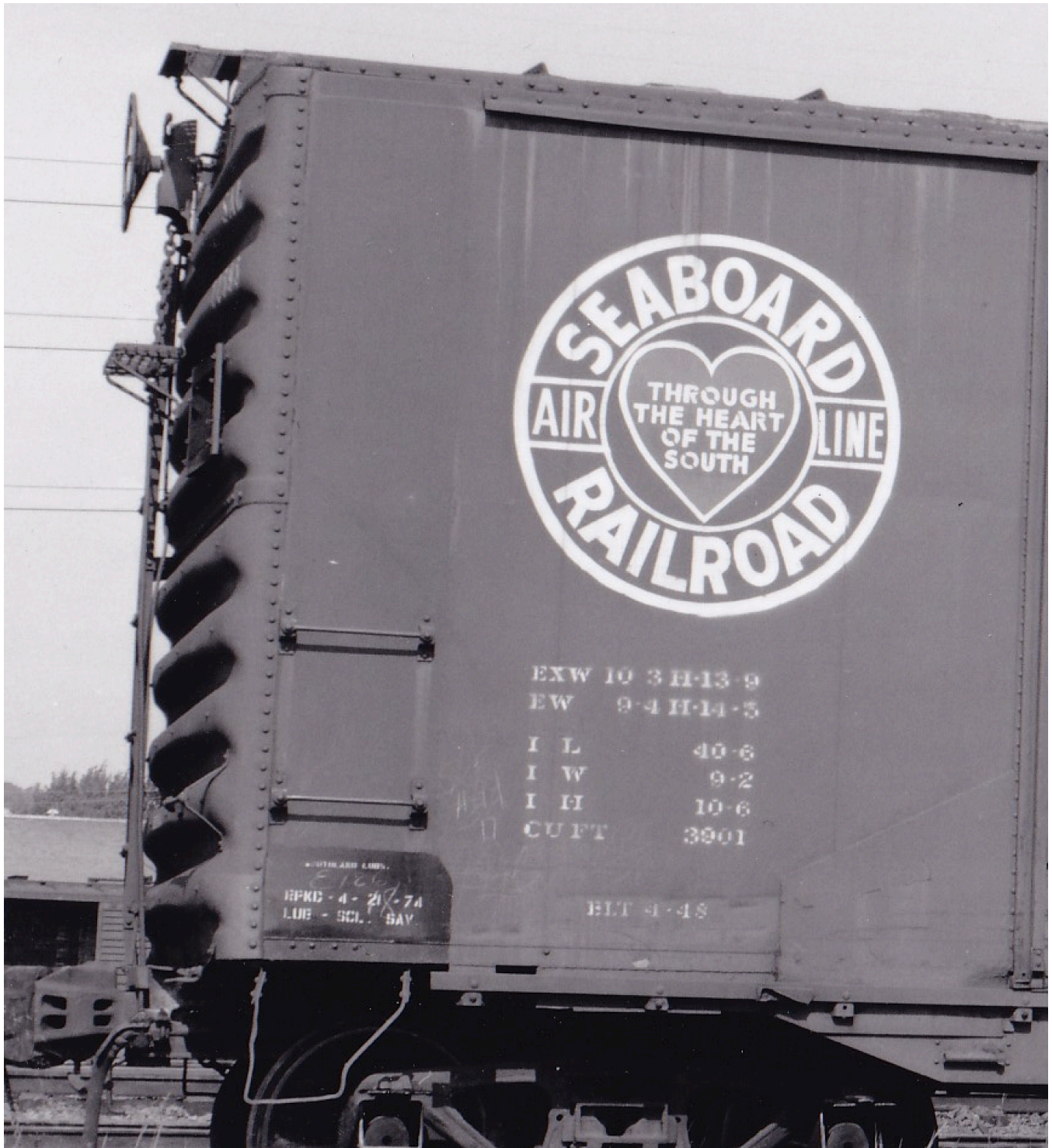
The B end image of SAL 22595 demonstrates the pre-1950-built end grab iron arrangement, the extended door track, and the brake gear arrangement. The Apex running board and brake step support and a high mount tack board can be seen in this view. In this post-1960 view, the addition of doorway gussets and a defect card holder can be viewed. The April 1974 Savannah, Georgia repack data is also clearly seen. (Bob's Photo)
