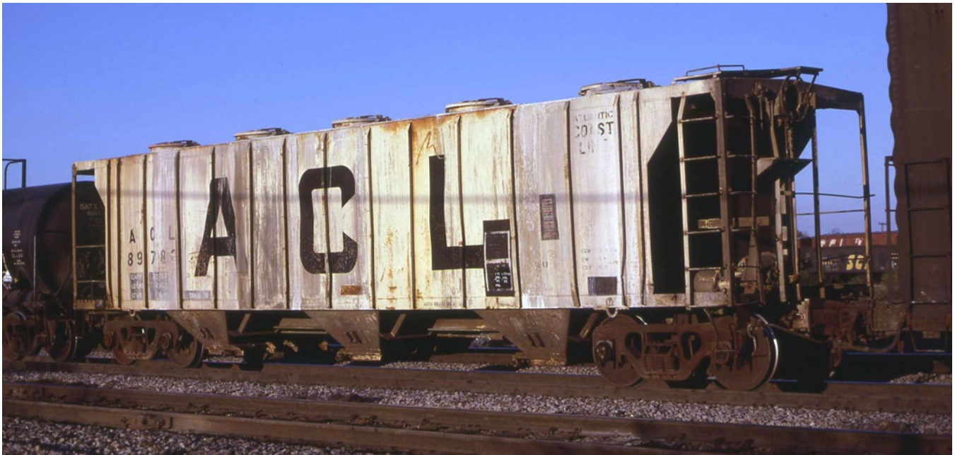
ACL 89780 was photographed in Hamlet, NC on April 5, 1980. The use of chemically resistant paints was used on later orders which prevented such paint failures. (Bob Graham photograph, Author's collection)
