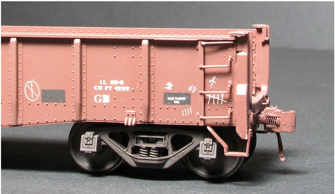
Photo 7: Tahoe Model Works TMW-210 70-ton ASF A-3 Ride Control solid bearing trucks are installed beneath the car to model the prototype trucks.
