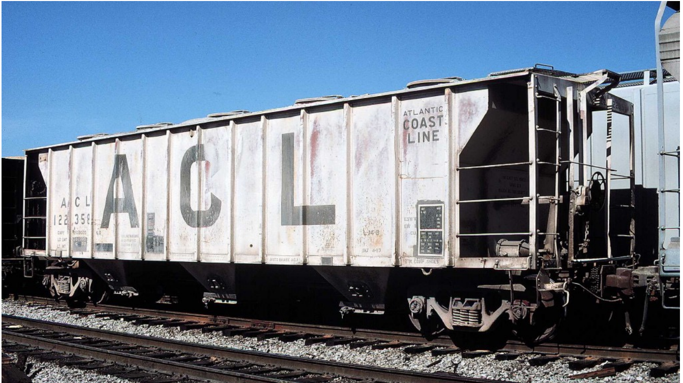
ACL 122358, a L-14-B class car, retains its original reporting marks, but has received additional stenciling and patched data. The low mounted brake wheel and extended running board are evident. (Bill Folsom photograph, Author's collection)
