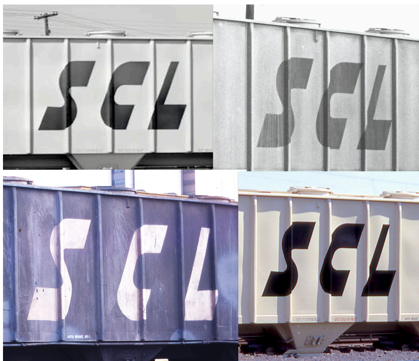
SCL 421575, is seen in the standardized cement service paint scheme typically applied to GATC Whalebelly pneumatic covered hoppers. A sister car, SCL 421241, was also painted in this scheme in 1974 which followed SCL lettering standards and utilized the 6' tall italicized letters equally spaced on the car side. Comparison to cars used in phosphate and feed service reveal a smaller variation is typically used for a vast majority of the repainted cars. (Larry Goolsby photograph)
