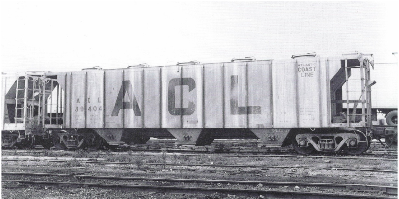
ACL 89404, seen in Lakeland, Florida on March 15, 1968. This car is loaded with 100-tons of processed phosphate and will be returned to a local facility where it reloaded with another shipment. (Bob's Photos)
