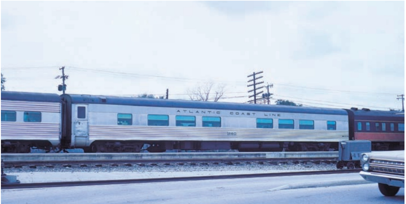
As contrast to the Seaboard Air Line purchased cars, ACL 260, a former NKP Plan 7600A example, shows the small detail variation between cars originally purchased by NKP. The fluting differed by an additional flute as compared to those cars originally purchased by C&O and later Seaboard. ACL 260 sits in St. Petersburg, Florida, on an unknown date. (Paul Coe photograph, Author's collection)
