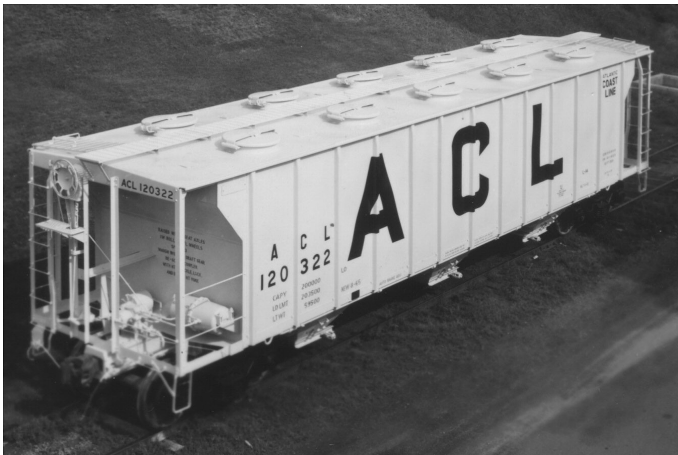
ACL 120322, a member of the L-14 series, is seen following construction in this builder's photo. The car was part of an 800-car order placed in 1965. (Pullman-Standard photograph, Jim Kinkaid collection)
