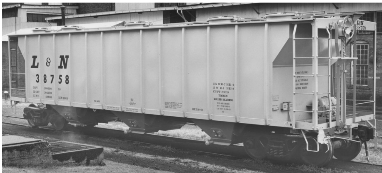
L&N 38758 was one of the earliest examples of the Pullman-Standard 2929 cubic foot design. The high mounted hand brake components can be seen in this B end view. Of note, the lack of a brake lever indicates these cars were equipped with truck mounted brakes. ( Pullman-Standard photographs, Jim Kinkaid collection )
