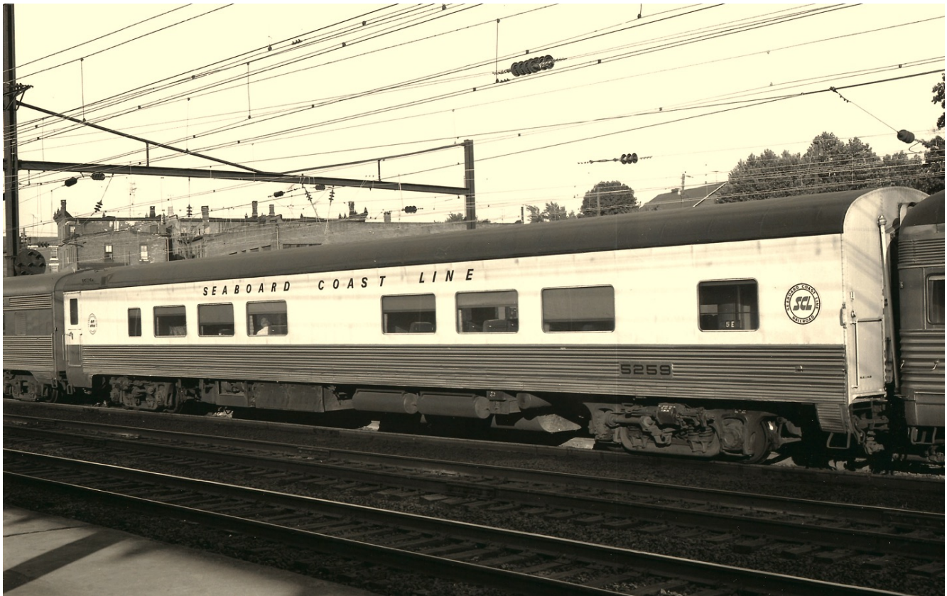
SCL 5259 is seen under the wires in PRR territory. The car, a former C&O Plan 7600 52-seat coach displays the unique appearance of these useful coaches. (Bob's Photo, Author's collection)
