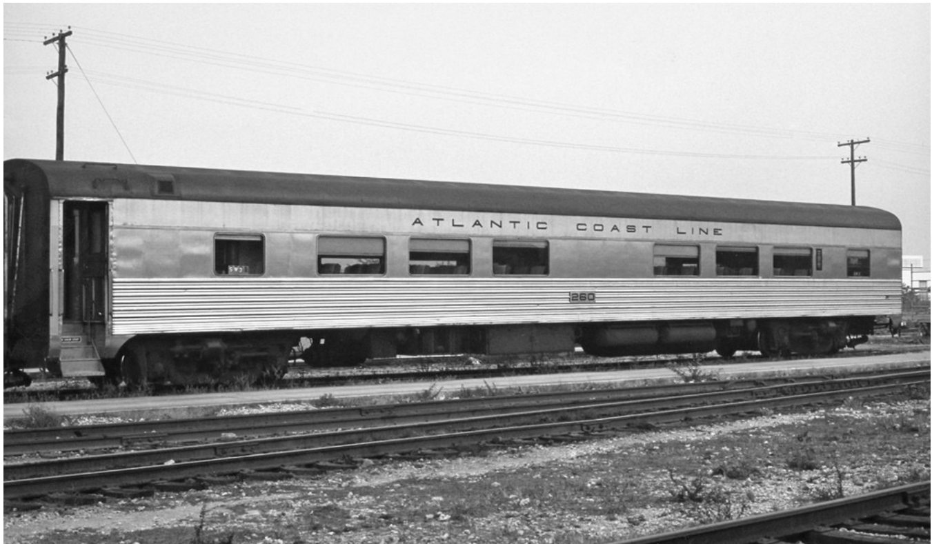
ACL 260, formerly Nickel Plate Road 100, was constructed by Pullman-Standard in 1950 to Plan 7600A. ACL 260 was modernized with the removal of the lower skirting and the upper band repainted using a metallic gray paint. (Robert Olesesski photograph, J. Brent MacGregor collection courtesy of RRPA)
