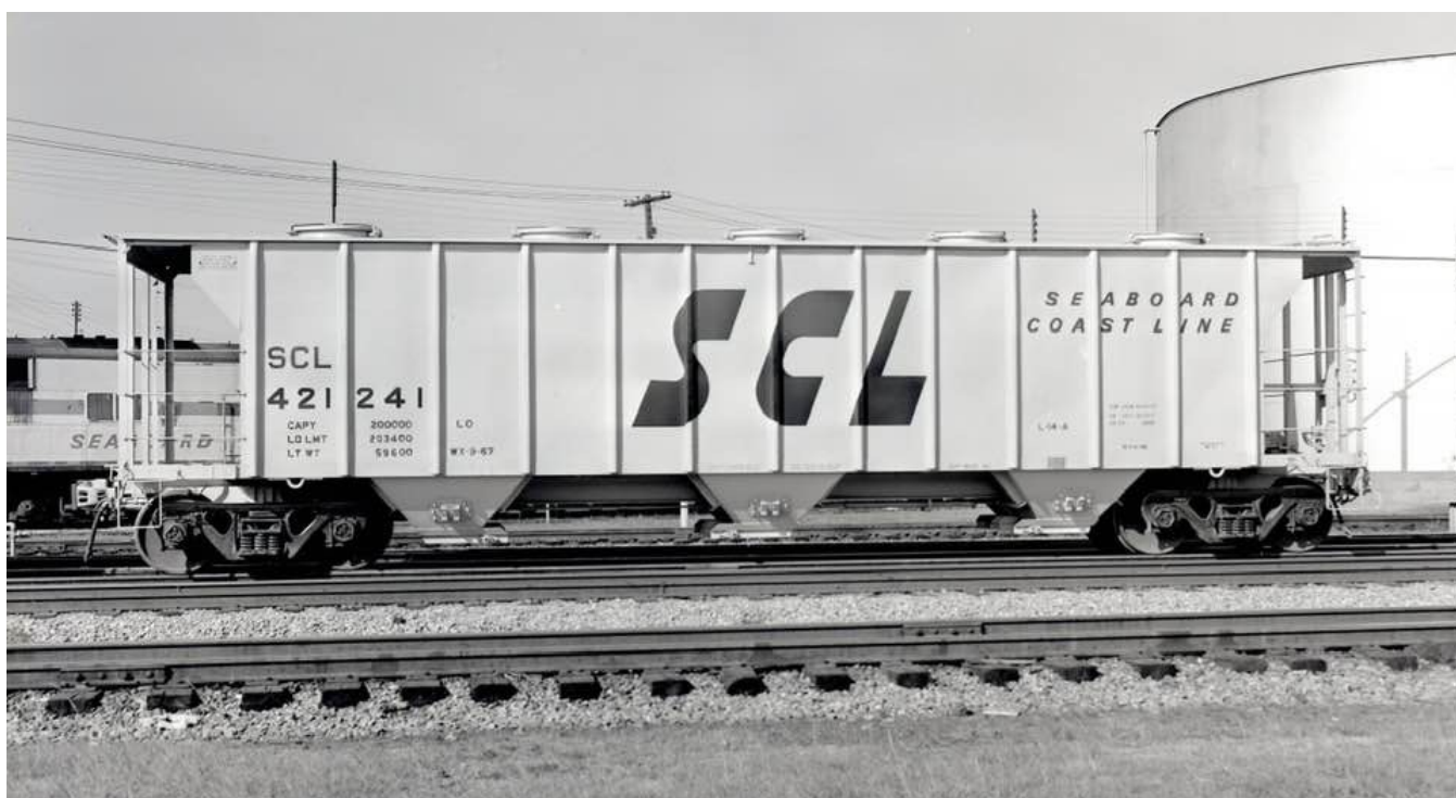
SCL 421241 has been freshly repainted in the Waycross shops in September 1967 as part of SCL's display train immediately following the SCL merger. The standard paint scheme of beige car color with black stenciling was utilized by ACL, SCL, and successors Seaboard System and CSX Transportation. (Warren Calloway photographs, Author's collection)
