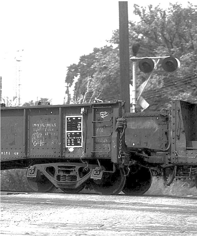
(Bottom page 10 and left) SAL 6521 is seen passing through Raliegh, NC on an unknown date. The reweigh stencil indicates the car is in SCL ownership and was last tested in March 1982. The build date of January 1949 is plainly visible and the Universal pump handbrake is seen in this B-end photograph. ( Warren Calloway photograph )
