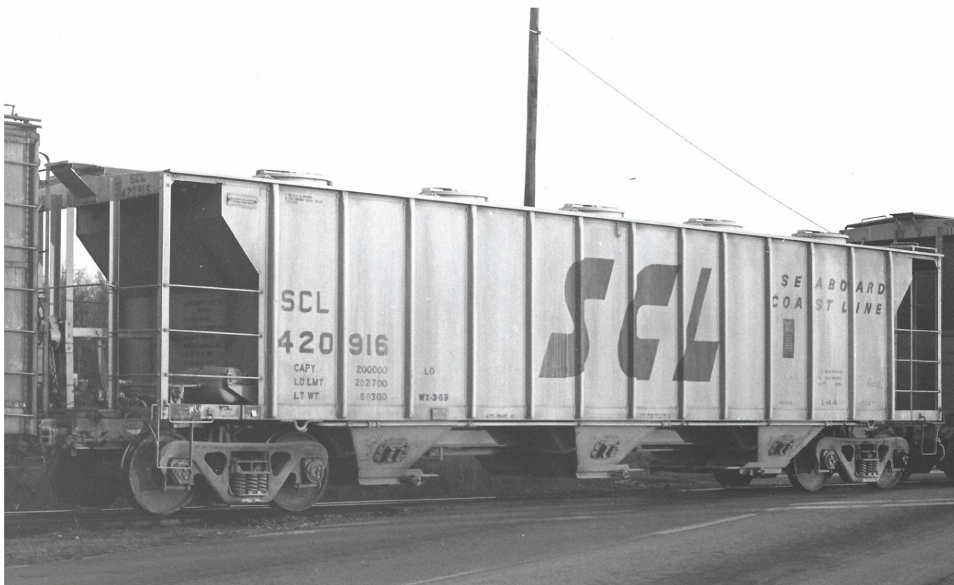
SCL 420916 is in Savannah, Georgia on December 21, 1970. Several 2929s were repainted as needed, however, most survived in their as-delivered paint given their recent construction just before the Seaboard Coast Line merger date on July 1, 1967. This car is a member of the SCL L-14-A class and provides an excellent in-service view of the SCL lettering applied. (C.L. Goolsby photograph, Author's collection)
