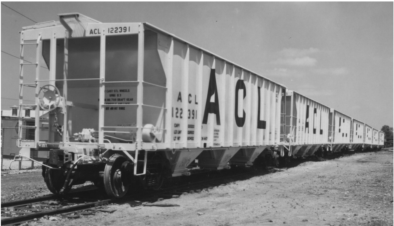
ACL 122391 is sitting with several additional examples of L-14-B 2929 covered hoppers. These cars were equipped with the extended running boards as seen in this view. (Pullman-Standard photographs, Jim Kinkaid collection)
