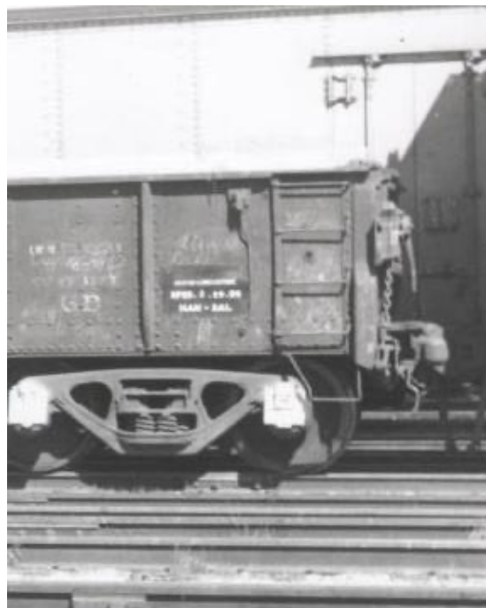
Photo 3: The exposed handbrake housing located on the B end of the SAL GB class gondolas. The housing is identified as a Universal Railway Devices 5825-B ratcheting pump handle type.
