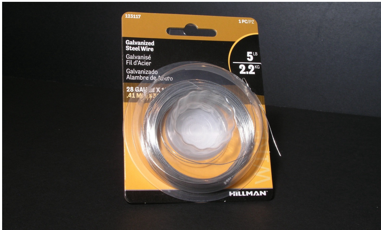
Photo 8: Hillman 28-gage galvanized steel wire used to create the rebar load.
