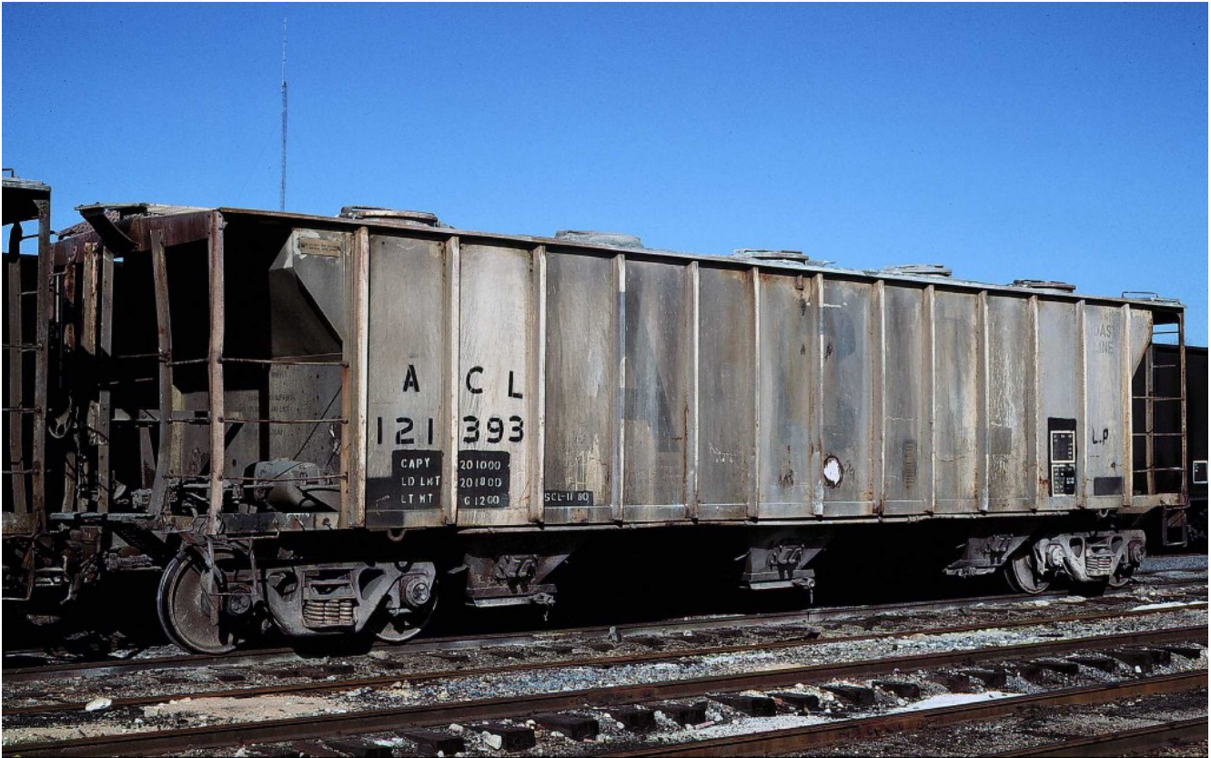
ACL 121393, a member of the L-14-B series sits in Atlanta, Georgia during the 1980s. The trust plate applied to the left slope sheet panel is present. The addition of reweigh data and a COTS panel along with years of lading and grime demonstrate how much use these cars saw. (Bill Folsom photograph, Author's collection)
