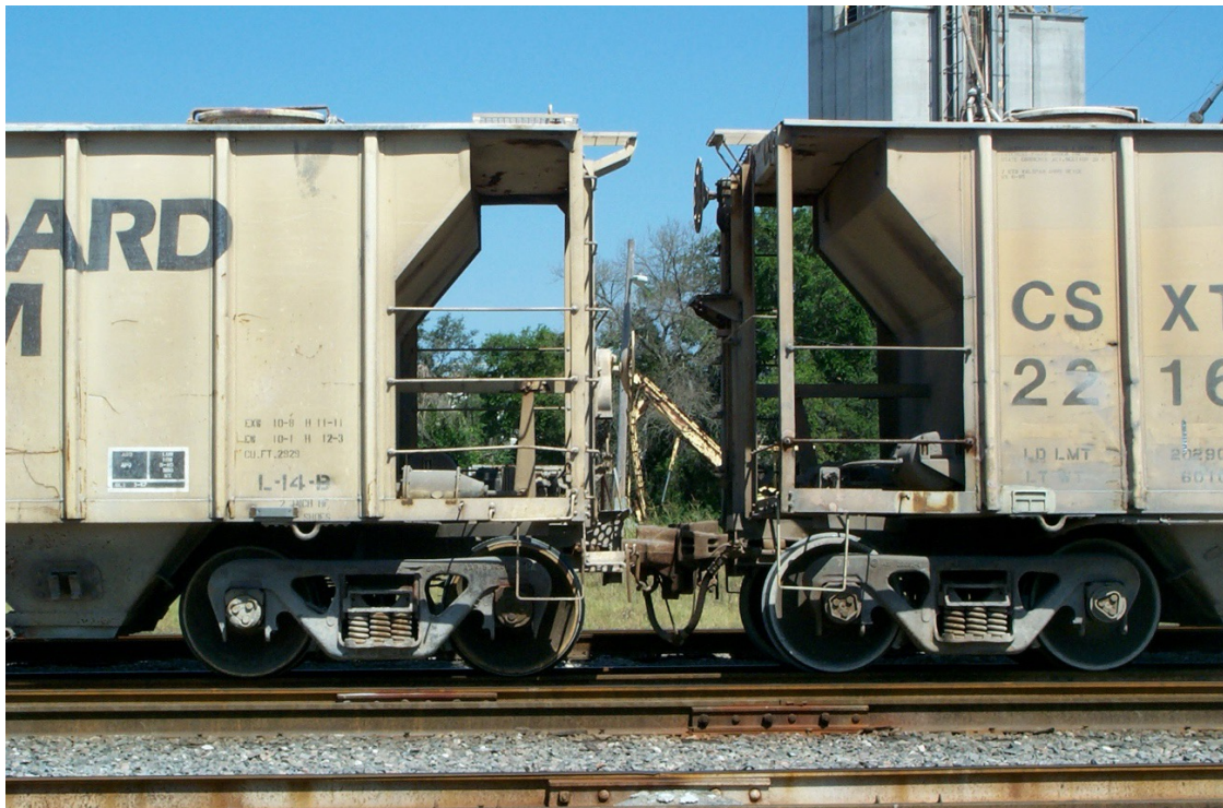
Seaboard System 222831 was photographed in Mulberry Yard on May 9, 2002. The car is a member of the L-14-B series, and is coupled to CSXT 221622, a member of the L-14 series. Note the differences in hand brake locations. (Author's photographs)
