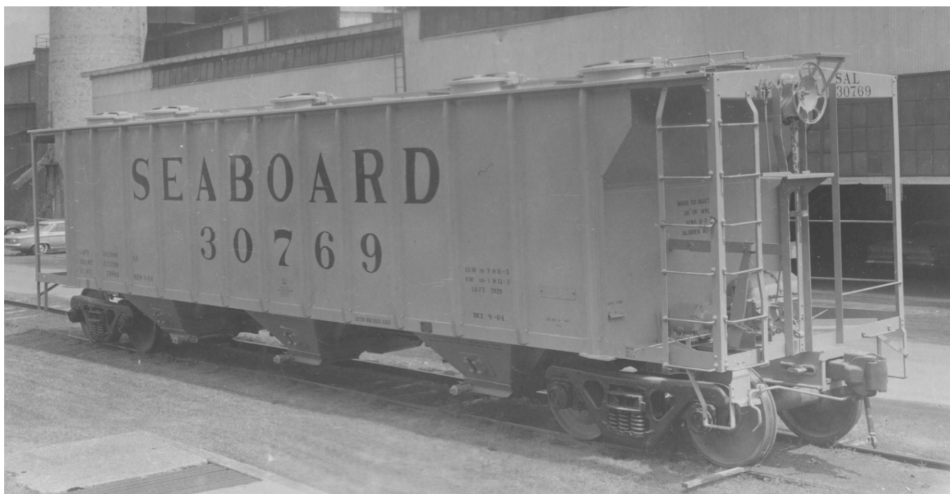
SAL 30769, a member of the initial 1964 order placed by Seaboard Air Line was unique with the offset 30" hatch spacing. This configuration was only applied to Lots 8917 and 8876. (Pullman-Standard photograph, Jim Kinkaid collection)
