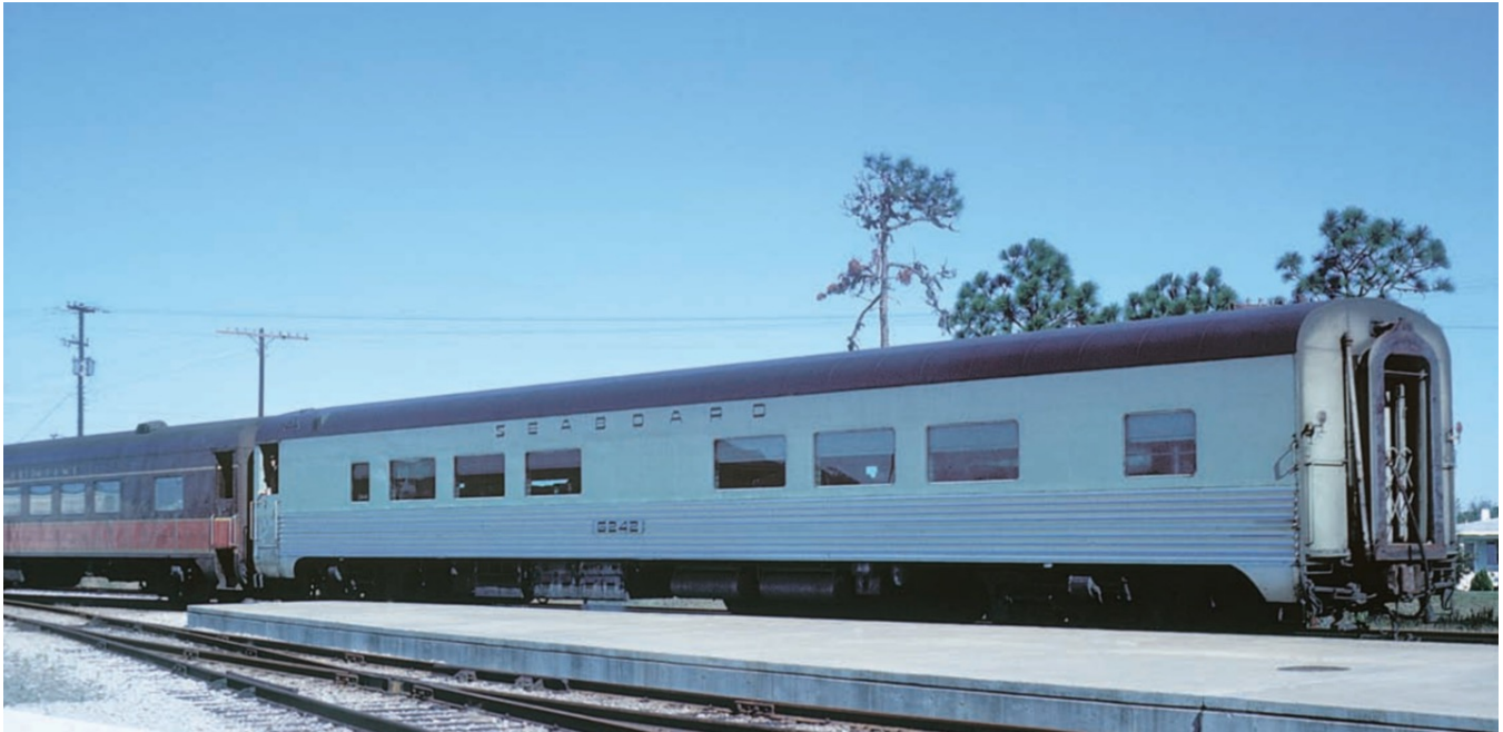
SAL 6242 sits at the St. Petersburg, Florida platform awaiting departure in December 1967. The Pullman-Standard Plan 7600 was purchased from C&O in June 1958 to supplement long-distance Seaboard Air Line Meteor and Star service. The car was repainted above the stainless-steel fluting using a metallic gray paint. (Paul Coe photograph, Author's collection)
