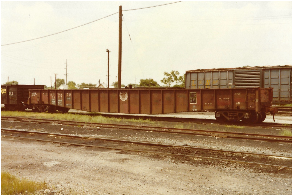
SAL 6527 was photographed after the application of a double COTS panel and lacking a drop end in 1984. (Stuart Thayer photograph, Author's collection)
