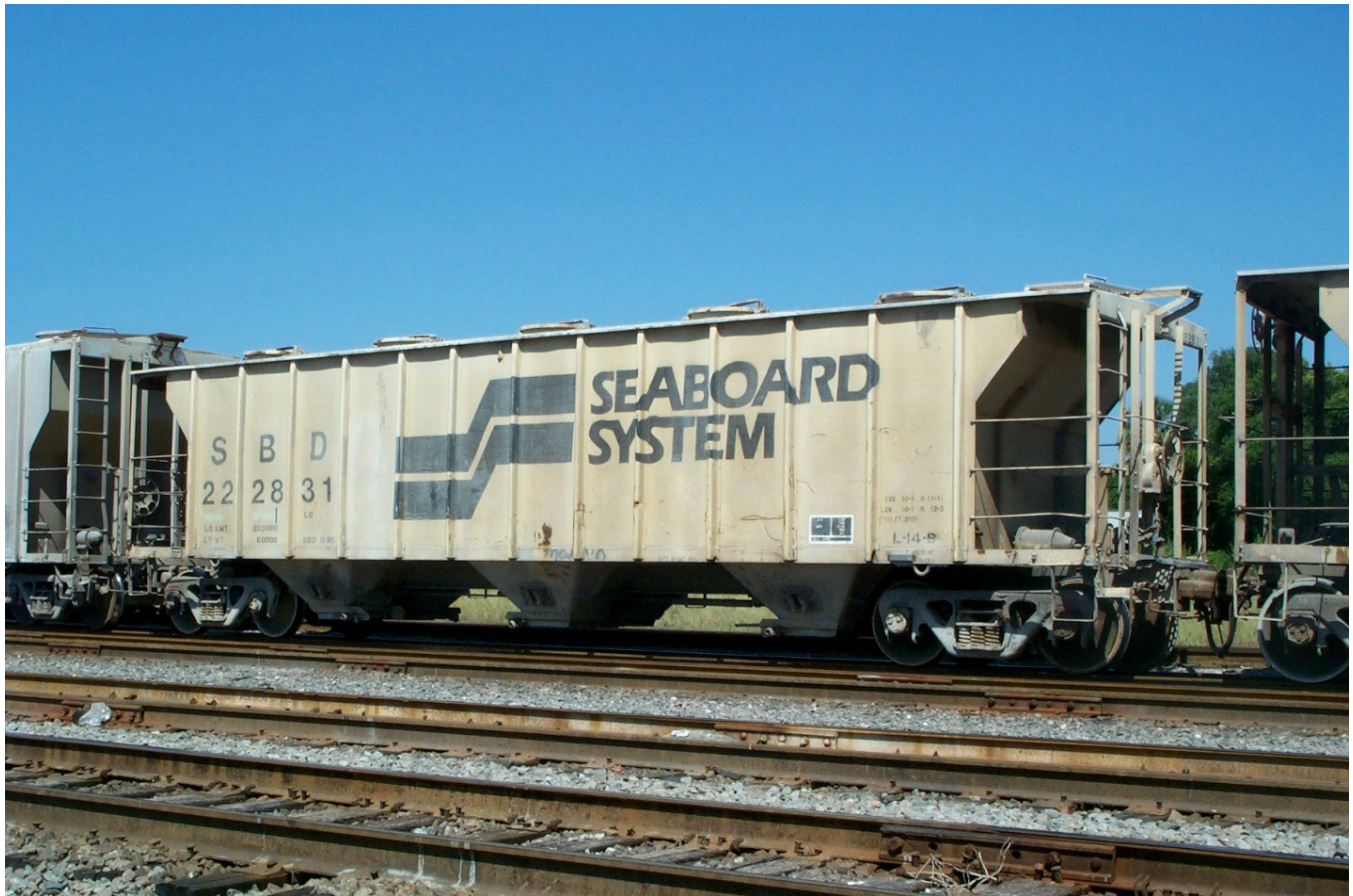
Seaboard System 222831 was photographed in Mulberry Yard on May 9, 2002. The car is a member of the L-14-B series, and is coupled to CSXT 221622, a member of the L-14 series. Note the differences in hand brake locations. (Author's photographs)
