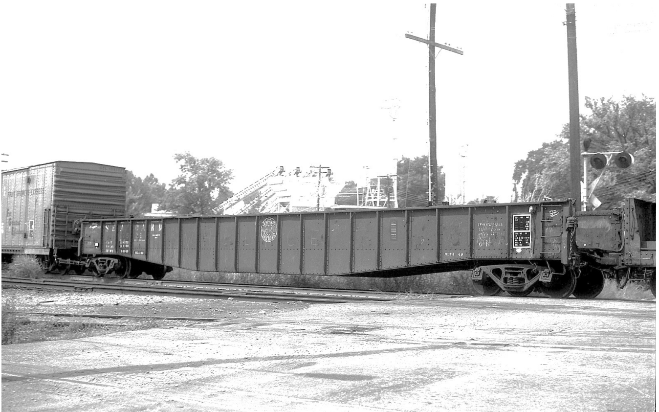
SAL 6548 is loaded with a high and wide load these gondolas were specially designed to handle. The use of idler flats on either side was typical when making special movements of freight. The car was photographed in Raleigh, NC on 09/04/1982. (Warren Calloway photograph)
