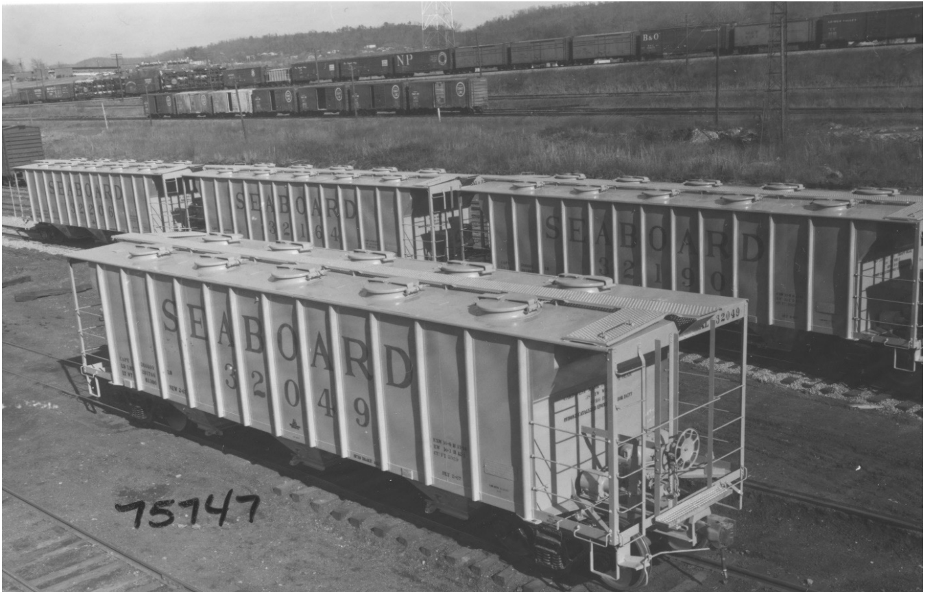
SAL 32049 with additional members of the order await final delivery in this builder's photograph view. The elevated view gives needed detail for modelers concerning the roof hatch spacing and B end brake configuration. (Pullman-Standard photograph, Jim Kinkaid collection)
