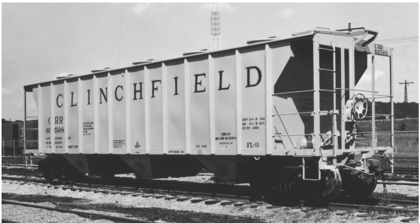
CRR 60568, an example of the FL11 series, constructed in May 1967. The differences seen from the FL10 series above include the lowered brake components, differing stirrup configuration, and an extended running board. (Pullman-Standard photographs, Jim Kinkaid collection)
