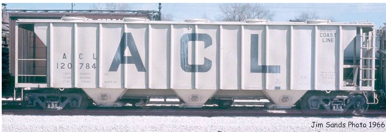
An in-service view of ACL 120784 is seen in Marshalltown, Iowa in 1966. The shipment of phosphate to farmers, Co-Ops, and fertilizer dealers throughout the United States enabled larger quantities to be transported without the necessity of bagging and shipment in boxcars as previously used. (Jim Sands photograph, courtesy of G. Elwood's Fallenflags.org)
