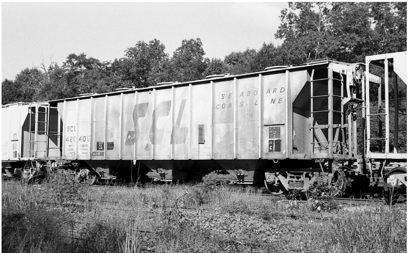
SCL 420405, a member of the L-14 series, and formerly ACL 120405, is found in train surrounded by ACF CH-29 two bay covered hoppers in Yemassee, South Carolina on August 10, 1985. This car was placed in dedicated cement service to Lehigh Portland Cement Company, in Lehigh, Florida. (Randy Chassereau photograph)
