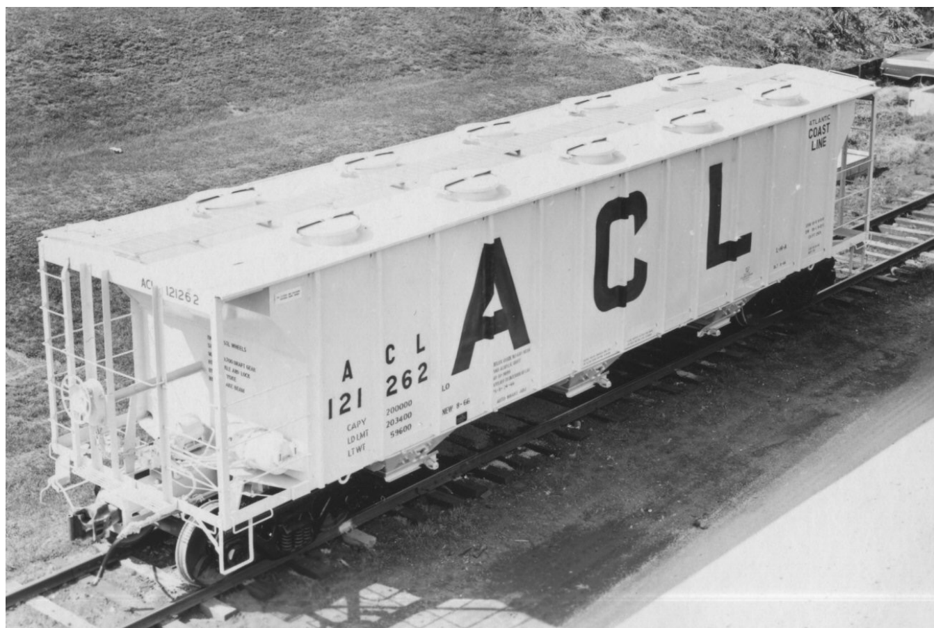
ACL 121262 was part of a 1,000-car order delivered in 1966, which was the largest order of the 2929 cubic foot covered hoppers delivered by Pullman-Standard. (Pullman-Standard photograph, Jim Kinkaid collection)
