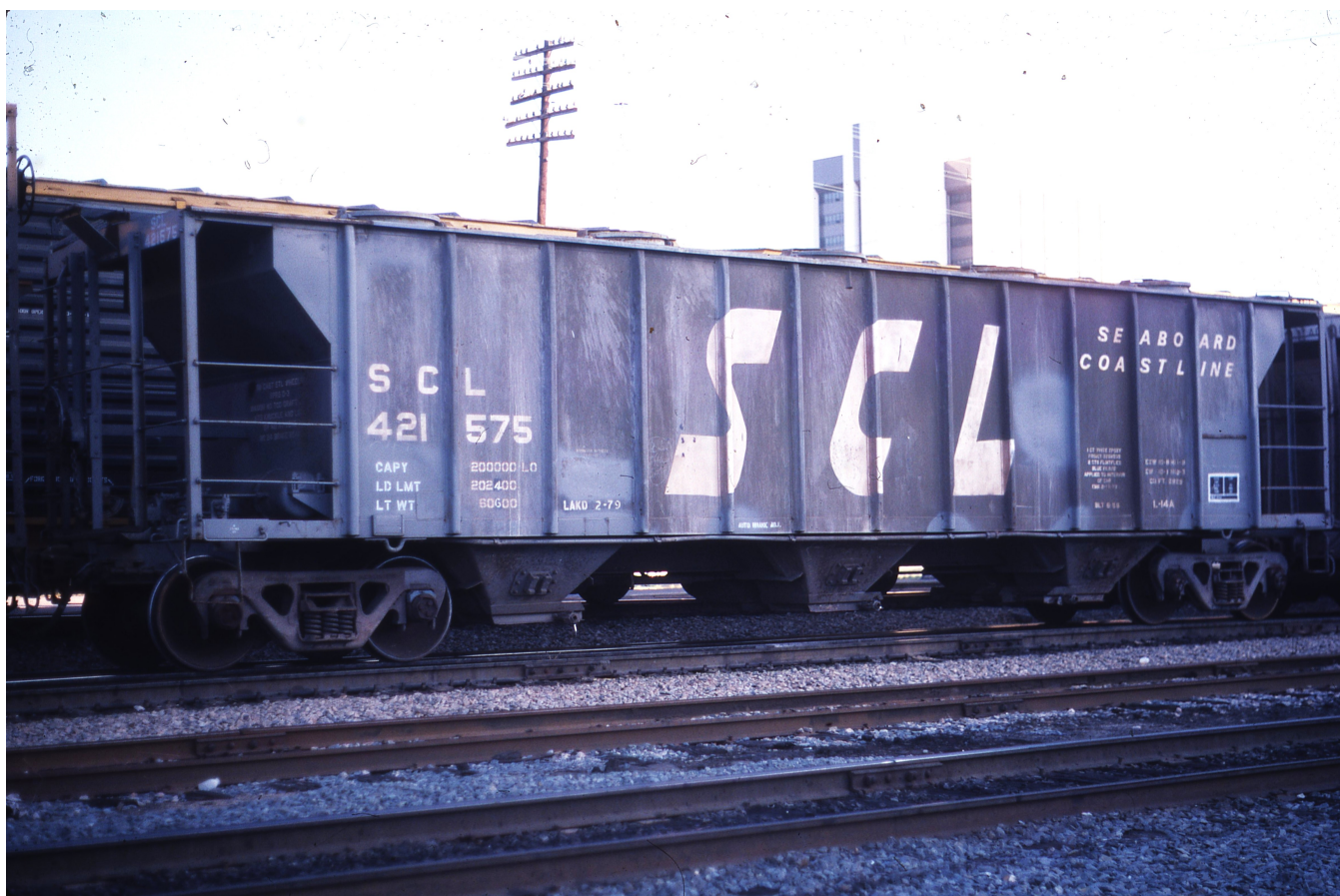
SCL 421575, is seen in the standardized cement service paint scheme typically applied to GATC Whalebelly pneumatic covered hoppers. A sister car, SCL 421241, was also painted in this scheme in 1974 which followed SCL lettering standards and utilized the 6' tall italicized letters equally spaced on the car side. Comparison to cars used in phosphate and feed service reveal a smaller variation is typically used for a vast majority of the repainted cars. (Larry Goolsby photograph)
