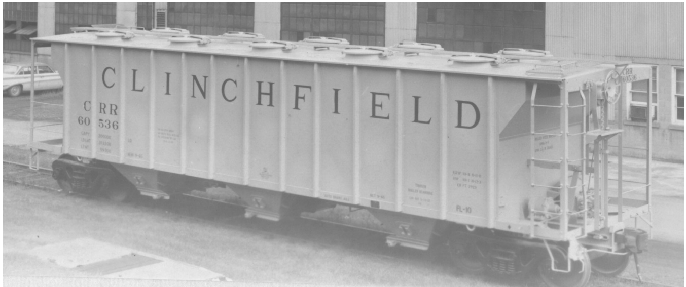
CRR 60536, an example of the FL10 class of 2929 cubic foot covered hoppers delivered to Clinchfield in September 1965. (Pullman-Standard photograph, Jim Kinkaid collection)
