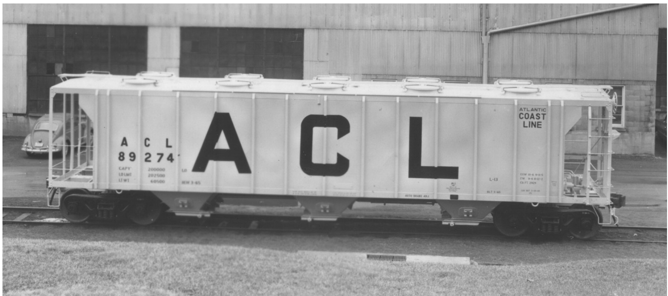
ACL 89274, is seen in Butler, Pennsylvania prior to delivery to owner Atlantic Coast Line. The L-13 series was not painted with chemically resistant paint which when seen in later years is likely the reasons for advanced deterioration of the car lettering and paint. (Pullman-Standard photograph, Jim Kinkaid collection)
