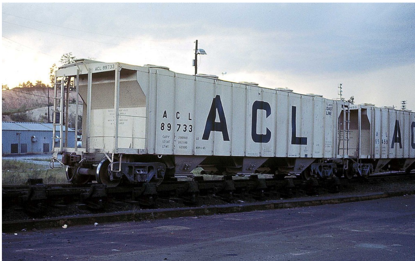
ACL 89733, a member of the 1965 built L-13 class showcases the unique double post configuration at the bolster and the lack of a non-overhanging roof. (Bill Folsom photograph, Author's Collection)
