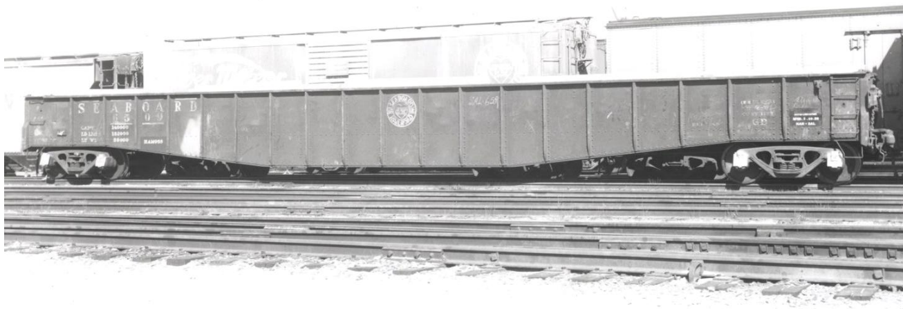
SAL 6509 sits in Seaboard's largest yard in Hamlet, NC. The use of yellow journals was not restricted to gondolas, but has also been seen on open hoppers, and denotes the use of specialized bearings. The repack date indicates it was repacked in Hamlet in September 1958. (Col. Chet McCoid photograph, Bob's Photo)
