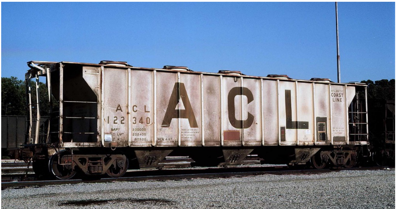
ACL 122340, another L-14-B series car, still showcases its 4-1967 build date and paint data. The ends have been bent likely due to the use heavy equipment to shove the car, a common issue on many covered hoppers. The car was once in dedicated service based on the presence of the yellow stencil, however, is likely in general service again due to the painted-over stenciling. (Bill Folsom photograph, Author's collection)
