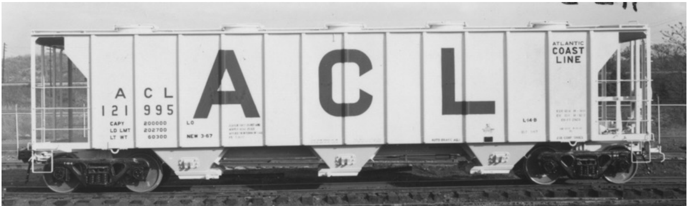
ACL 121995, a member of the L-14-B series, displays the unique reporting marks and number type face applied to this order delivered in 1967. (Pullman-Standard photographs, Jim Kinkaid collection)
